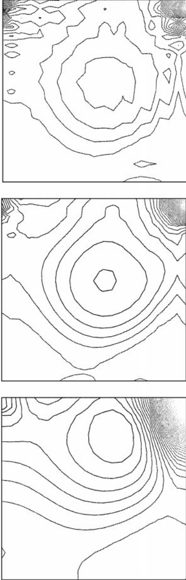
FIG. 1. Pressure contours for the cavity flow-problem using the first-order scheme. From the top to the bottom: \delta t = 0.1 \delta t_{\text{crit}} , \delta t = \delta t_{\text{crit}} , and \delta t = 1.0 .
